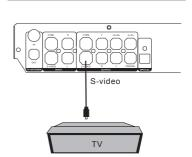
Connect your recorder with the S-Video cable, if the TV has an S-Video input. Do not connect the vellow video cable if using the S-Video cable
